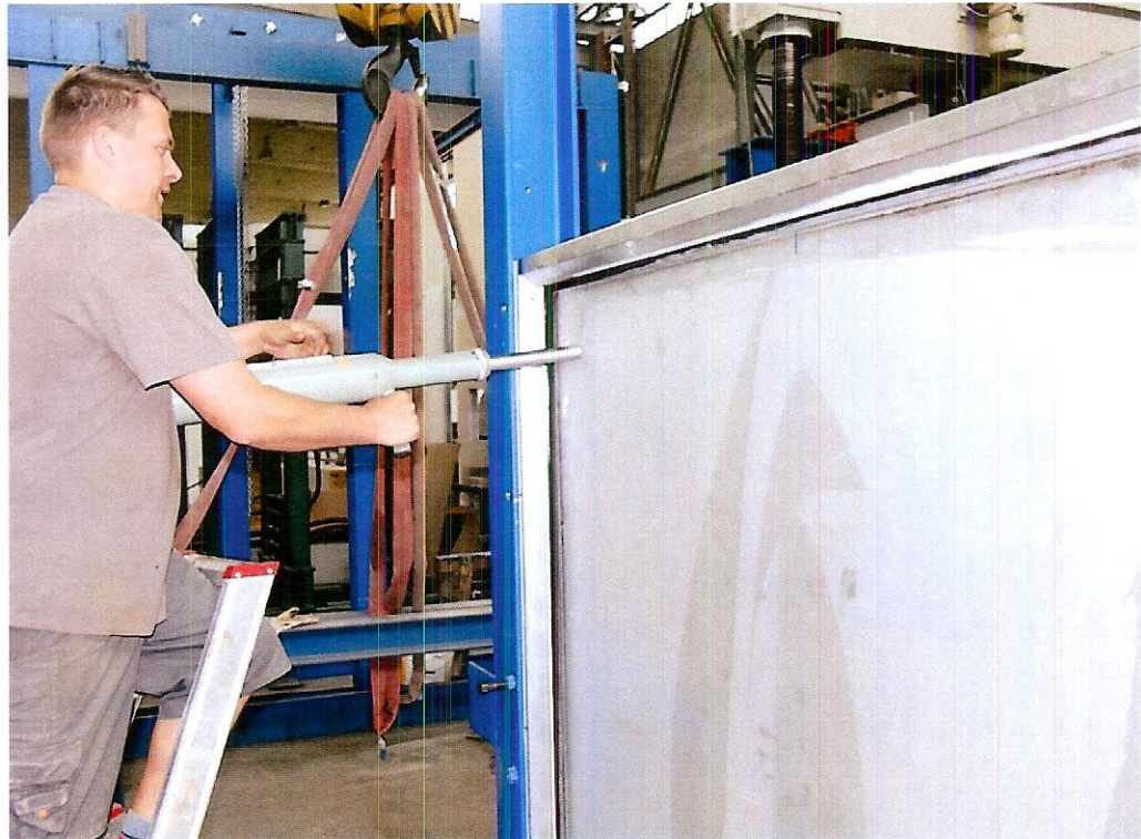
Figure A1-1: test of the PMMA-panel in the area of one corner of the test surface (point 1)
