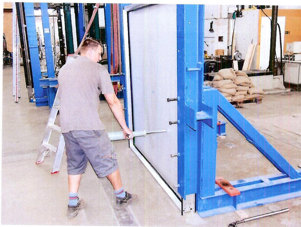
Figure A1-3: test of the PMMA-panel at another point selected at random within the test surface (point 3)
