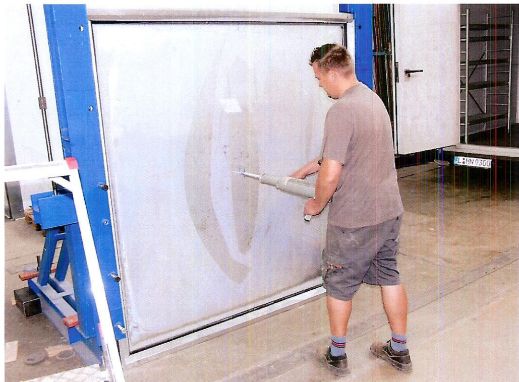
Figure A1-2: test of the PMMA-panel in the middle area of the test surface (point 2)
